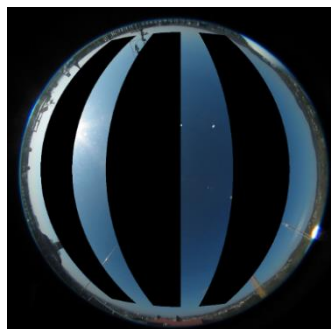
Fig. 1. Example of an edited fisheye photograph showing 3 rows of APV modules
