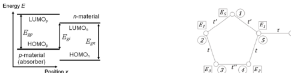
Fig. 1: Relative LUMO, HOMO energy levels of donor and acceptor materials and interpretation of relationship (Minnaert and Burgelman, 2007) and the Hubbard model of polythiophene (Gulácsi, 2013; Farchioni and Grosso, 2011)
