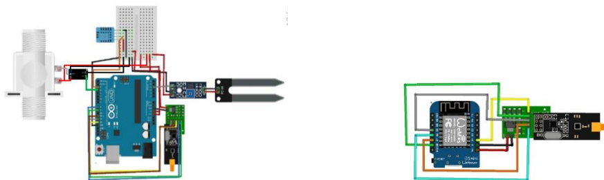
Fig. 1. Wiring diagram of the device with nRF24L01 module, Transmitter & Receiver
