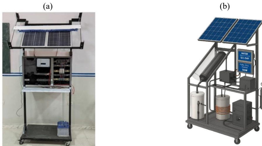
Fig 1. Intelligent solar energy systems: (a) System implementation (b) 3D design of IoT-Enabled hybrid PV-CPC
