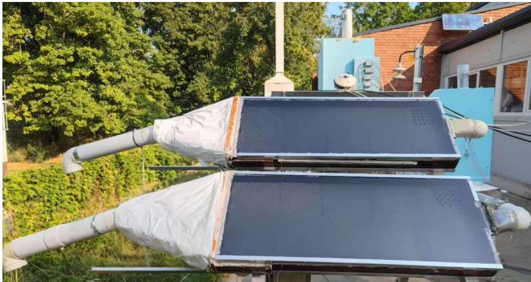
Fig. 1. The experiment setup for solar drying
