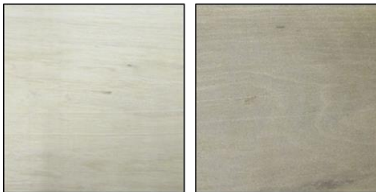
Colour change as a result of acetylation on hornbeam wood (left: untreated; right: acetylated)
